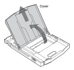
**3** Move the paper guides (vertical and horizontal) to the ends.
